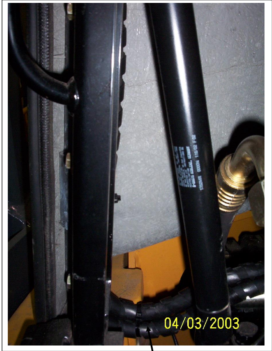
5/16" hose and 13/32" hose at the engine hood pivot point
