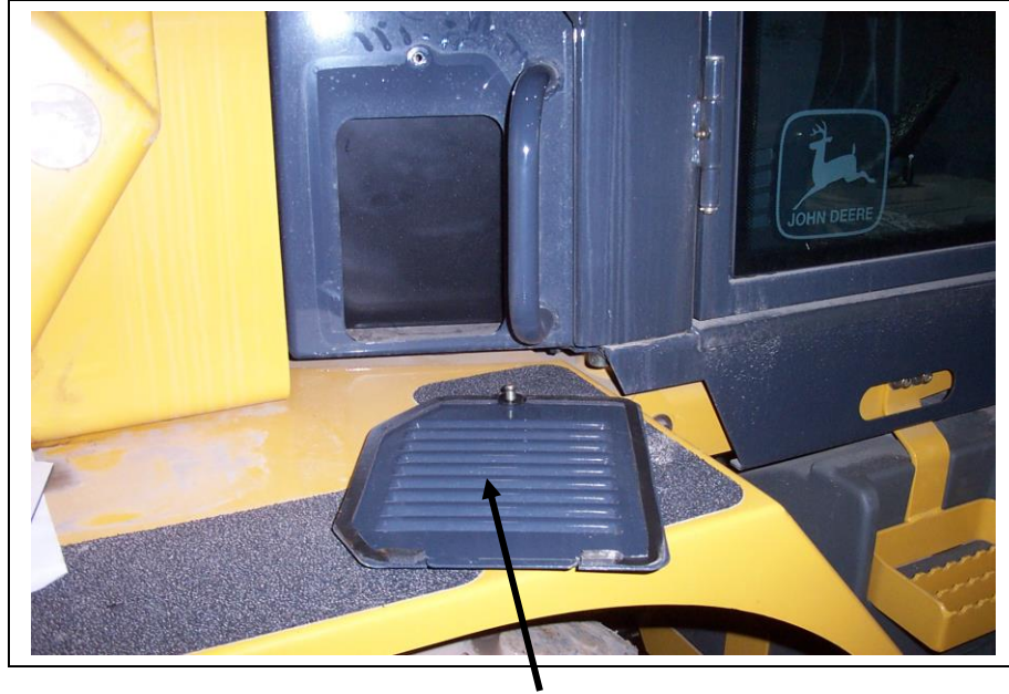
Outside air intake louvered door off.
