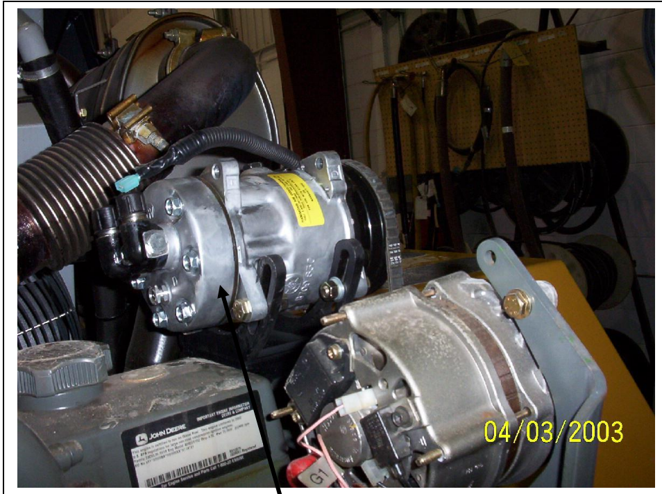
Compressor in place on the mount bracket
