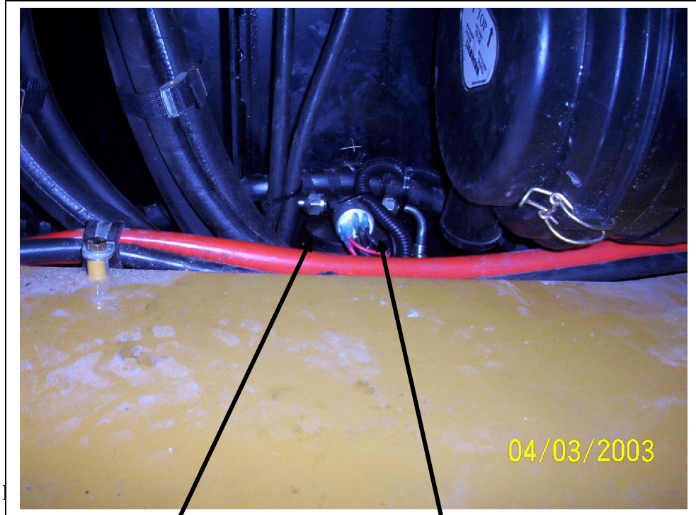
Trinary switch for compressor and hydraulic fan override for the condenser.
