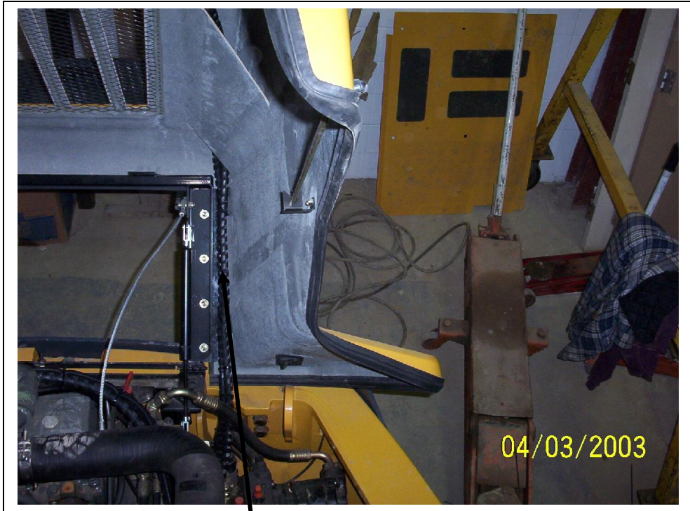
5/16" hose and 13/32" hose running down the inside of the engine hood to the pivot point of the hood.
