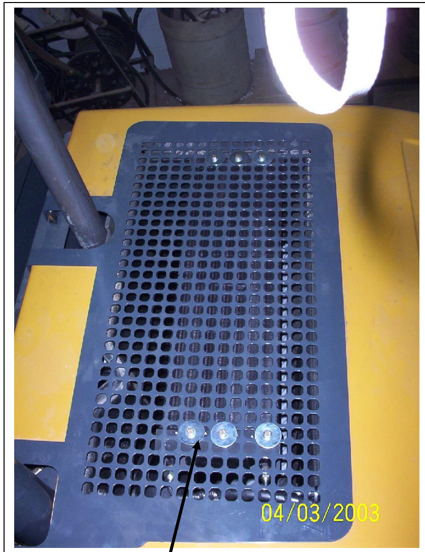
Condenser in place and bolted down through the radiator air intake screen. Use the 1/4" hardware and fender washers.
